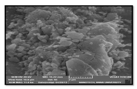
Figure.6 SEM Image of Titanium Dioxide Particles
