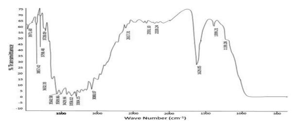
Figure 4. FTIR spectra of TiO2
