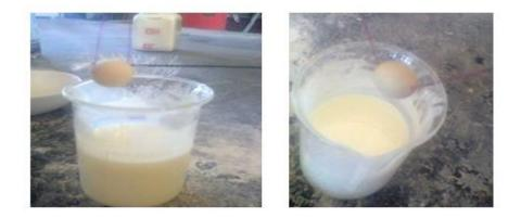
Figure. 3 Coating of Titanium Dioxide Gel Over Clay Pellet
