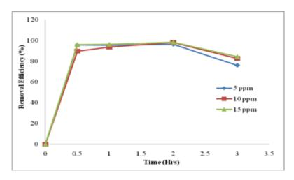
Figure.9. Variation of removal efficiency of lead with respect to time
