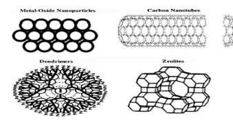
Figure 1. Selected nanomaterials currently being evaluated as functional materials for water purification (Courtesy: Savage and Diallo 2005)
