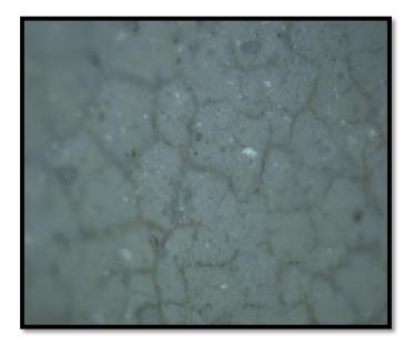
Figure. 5 Optical Microscope Image of Titanium dioxide Coated Clay Pellet Surface
