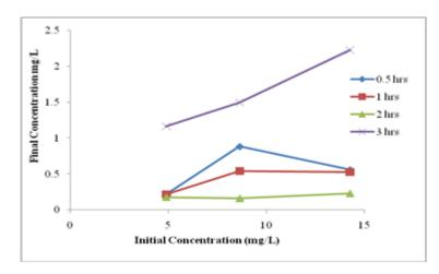
Figure.8. Variation of final concentration of lead with respect to initial concentration of lead
