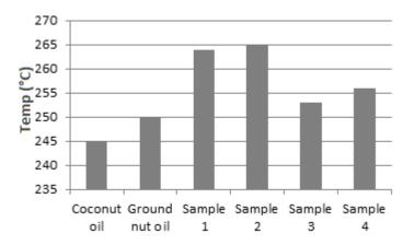
Figure 2: Flash point determination of prepared samples and base oil
