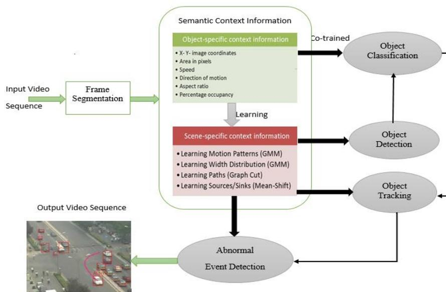
Figure 1: Proposed framework of Intelligent Video Surveillance System
