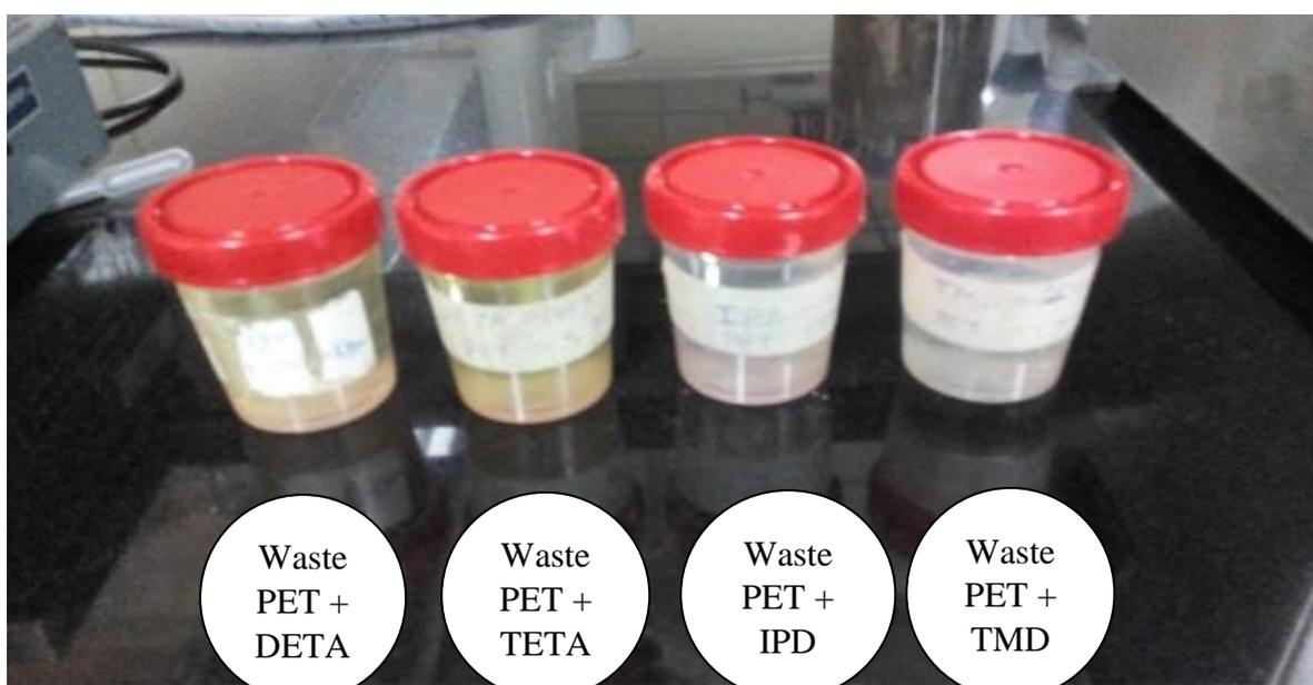
Fig.2 Dissolve the waste PET plastic pieces into Di ethylene triamine and Triethylene tetramine, Trimethyl, hexamethylene diamine, Isophoron diamine
