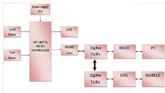
**Figure 4: Block diagram of pic microcontroller**
