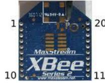
Figure 5: ZigBee module of 802.14.5
