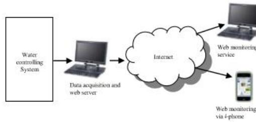
**Figure 2: Water level monitoring network**
