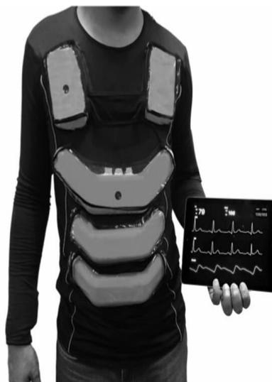
Prototype of wearable vital signs monitor.
