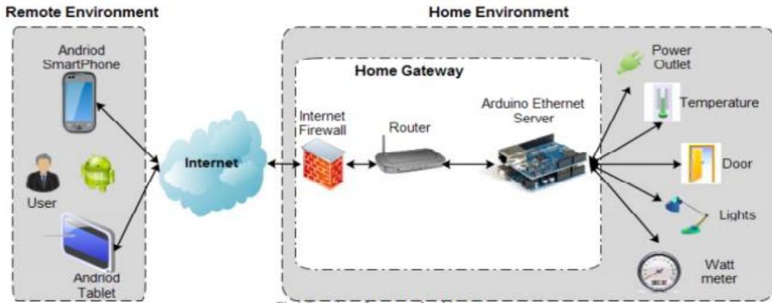
Fig.1 Overview of conceptual architecture.
