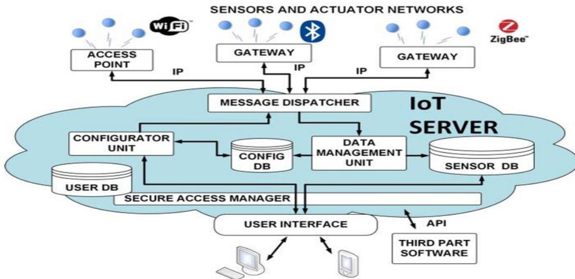
Figure 6: Block diagram of the internet of things platform supports in-home smart grid
