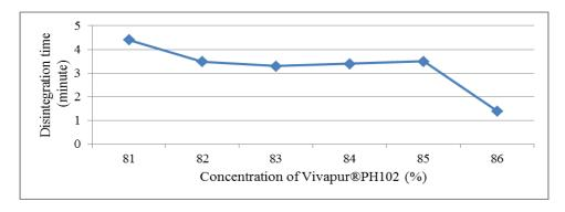
Fig.1 Correlation between Vivapur®PH102 concentration and disintegration time
