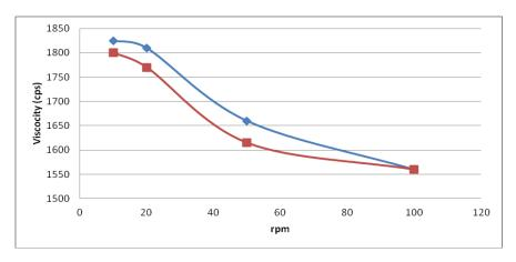
Figure 2. Rheogram of microemulsion gel (upward/backward curve)
