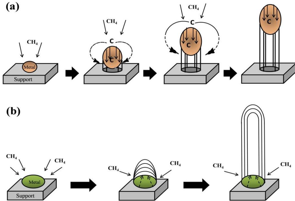
Figure 2: Growth mechanism of MWCNTs
