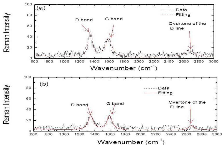
figure 3: Raman spectra of the prepared MWCNTs over (a) Fe-Mo catalyst, and (b) Ni-Mo catalyst.
