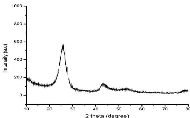
Figure 4: XRD pattern of the prepared MWCNTs over Fe-Mo catalyst
