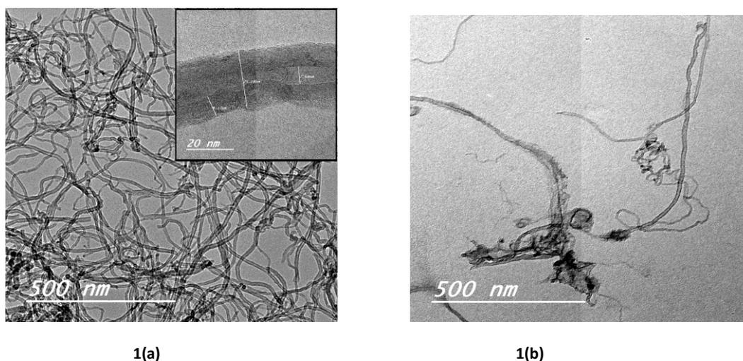
Figure 1: TEM images of the prepared MWCNTs over (a) Fe-Mo catalyst, and (b) Ni-Mo catalyst.
