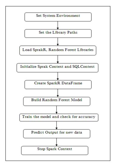
Fig 2: Control Flow Diagram of RF Modelling
