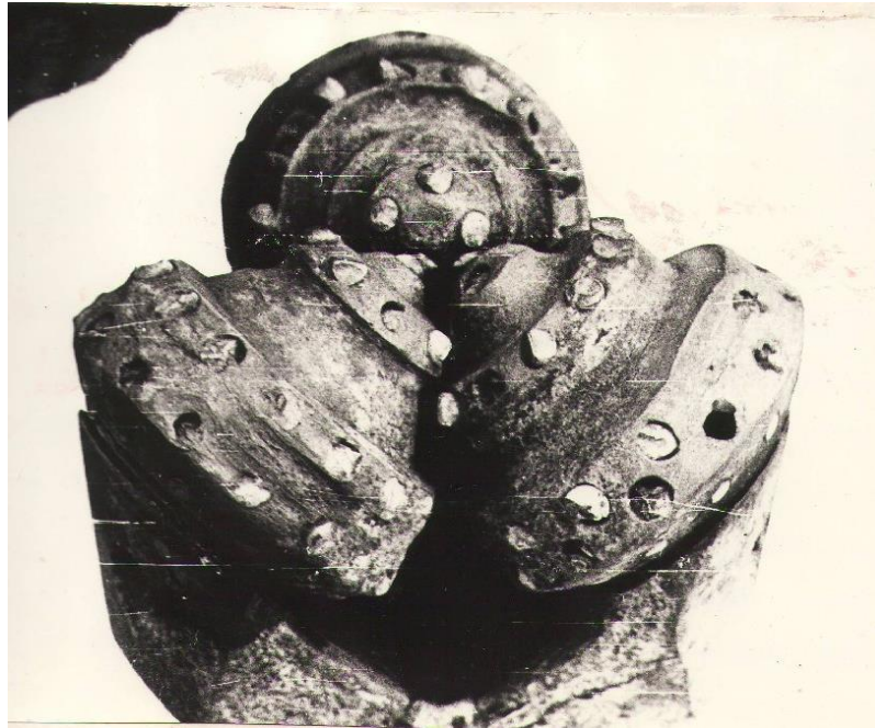
Figure 4. Typical destruction cases of cutting structure for worked off bits Ш215, 9TK3-ЦБ-3
