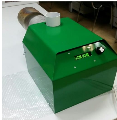
Figure 2. The prototype of the experimental burner with hardware-software complex of control automation for investigation tests conduction.
