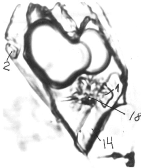
Fig.5. Multiphase of the fluid inclusion in skapolite; 1-Galit; 2-carnallite; 14-quartz; 18-mineral № 18. Increase of 900
