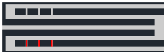
Fig. 4. Elastic suspension of the inertial mass
