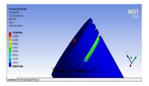
Fig: 5.3 Heat flux analysis on proposed Piston Face
