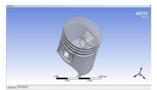
Fig: 4.1 3D Model of Piston's Surface
