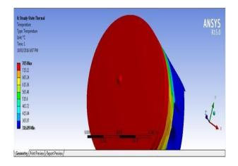
Fig: 4.5 Temperature analysis on existing Piston Face
