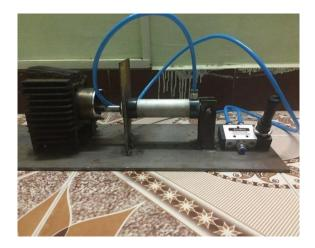
Fig: 6.1 Prototype of Hard chromium coated cylinder and piston assembly
