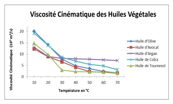
Figure 2: Kinematic viscosity of the different vegetable oils
