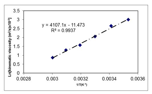
Figure 5: Dependence of Ln(viscosity) versus 1/T of olive oil.
