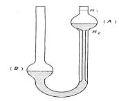
Figure 1: Osswald viscosimeter
