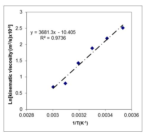
Figure 4: Dependence of Ln(viscosity) versus 1/T of avocado oil.
