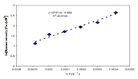
Figure 6: Dependence of Ln(viscosity) versus 1/T of rapeseed oil.
