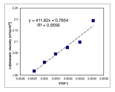
Figure 3: Dependence of Ln (viscosity) versus 1/T of argan oil.
