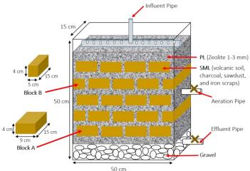
Figure 1: Design of MSL system
