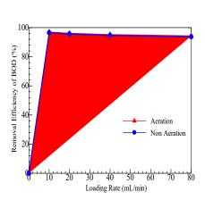
Figure 4: Removal efficiency of BOD
