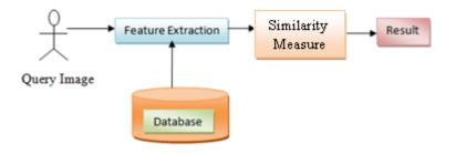
Figure 1.Block Diagram of CBIR
