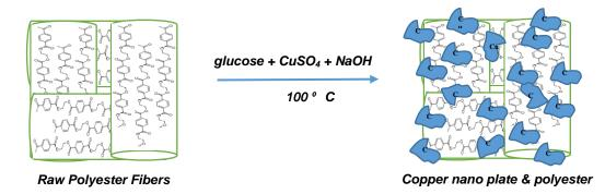
Figure 1: Polyester fabric finished with copper nano plate
