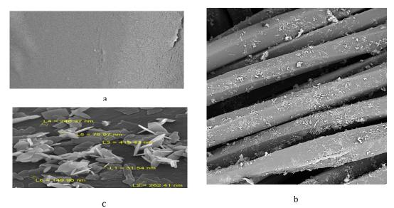
Figure 6: SEM images of different fabric samples: a) raw with 20000X, b) finished with nano copper 1000X, c) finished with nano copper 20000X,
