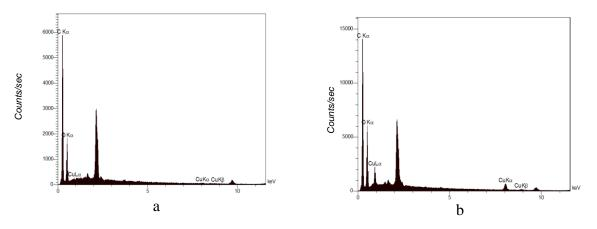
Figure 7: EDX patterns of: a) raw and b) modified polyester with copper nano plates
