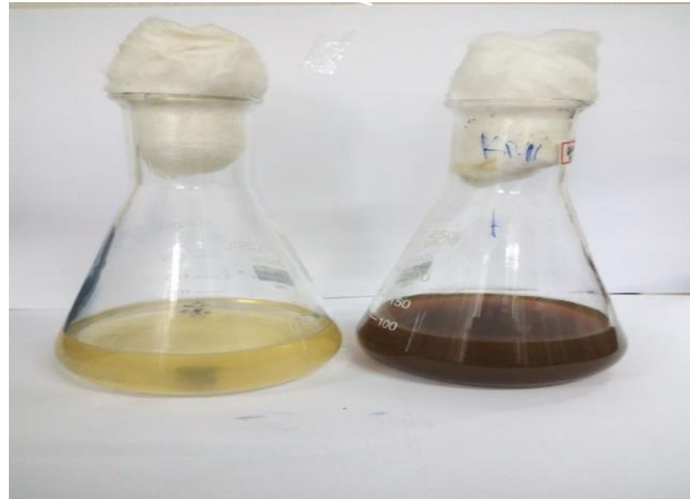
Figure 1: Synthesis of Silver nanoparticles (a) Bennet broth with AgNO 3 (b) Bio reduction of silver ions by streptomyces sp.KN11
