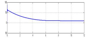
Fig. 6. Armature Current of Shunt Motor
