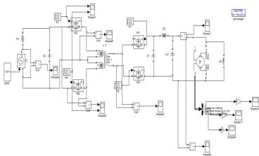
Fig. 2. Simulation circuit of Solar Based DC-DC Converter for Shunt Motor Application
