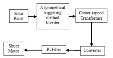
Fig. 1. Solar Based DC-DC Converter for Shunt Motor Application
