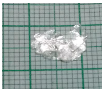
Fig.1 Photograph of grown LIDNV crystal
