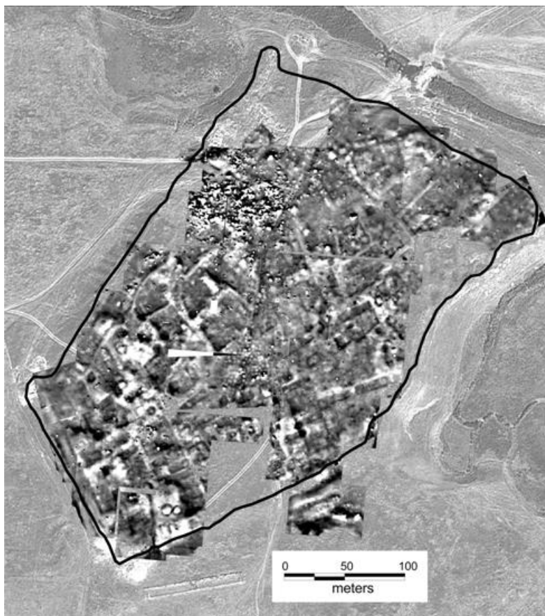
Figure 2. Map of anomalies of magnetic field on the hillfort “Belinskoye” obtained from a magnetic survey 2007-2012.
