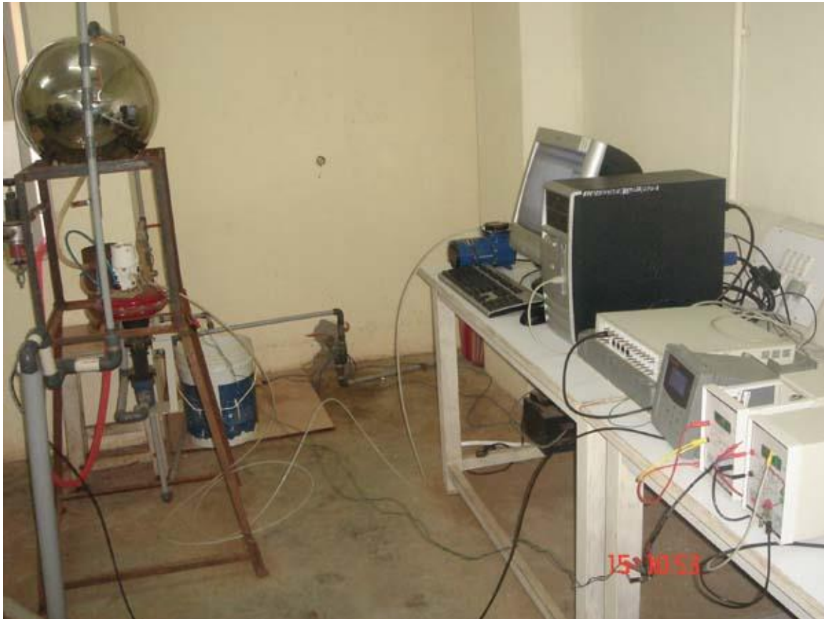
Figure 1 Real time Experimental setup for conductivity measurement
