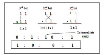
Fig 3 b. Binary Multiplication Illustration of Vedic technique.
