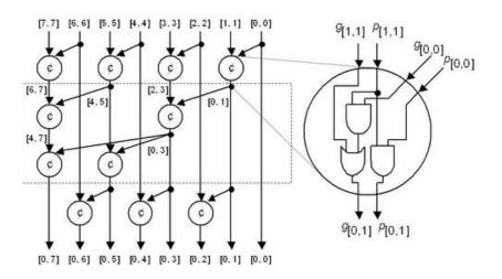
Fig 5. bit Brent Kung Adder network
