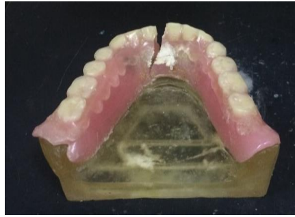
Fig 3: The experimental denture under load applicator of the universal testing machine, (b) denture fracture
