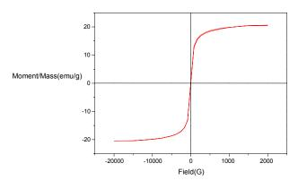
Fig (5): hysteresis curve of starch Fe<sub>3</sub>O<sub>4</sub>.
