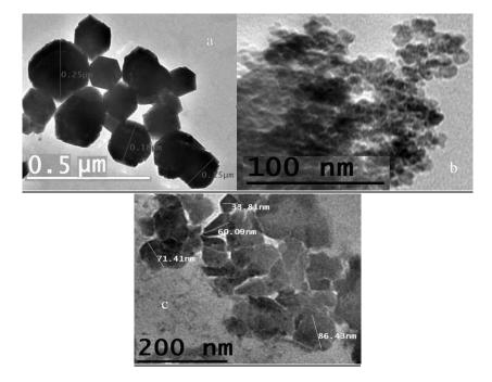
Fig (3): TEM images of stained native starch (a), unstained starch Fe<sub>3</sub>O<sub>4</sub> (b) and stained starch Fe<sub>3</sub>O<sub>4</sub>(c).
