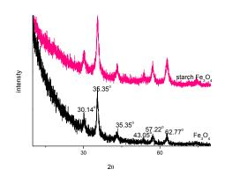
Fig (4): the XRD patterns of pure Fe<sub>3</sub>O<sub>4</sub>, starch Fe<sub>3</sub>O<sub>4</sub>.
