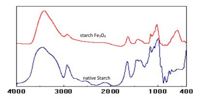
Fig (1): FTIR spectra of native starch and starch  $Fe_3O_4$  nanoparticle
