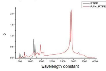
Figure 3: IR absorption spectra of PTFE: lower - PTFE top - membrane PTFE-PANI [7]
