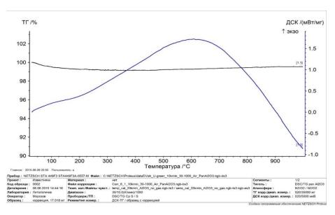
Figure 5: The results of thermoanalysis of CW. 1 – the curve of differential thermoanalysis, 2 – the curve of thermogravimetry.
