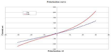
Figure 3: Potentiodynamic polarization curves, characterizing steel behavior 08 kp in contact with extract of CW
