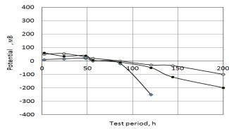
Figure 2: Kinetics of corrosive potential of aqueous extracts RFP (1); EW (2); CW (3)
