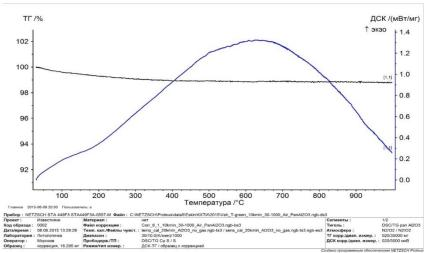
Figure 4: The results of thermoanalysis of FW. 1 – the curve of differential thermoanalysis, 2 – the curve of thermogravimetry,
