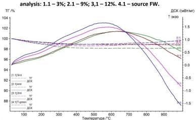
Figure 7: The results of thermal analysis of the mixtures of CW and zinc oxide. The curves of differential thermal analysis: 1.1 - 3%; 2.1 - 9%; 3.1 - 12%. 4.1 - source CW.
