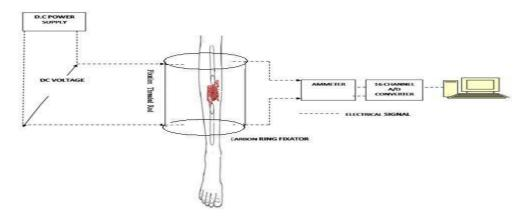
Figure 2: Experimental set-up for fracture healing model analysis
