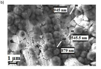
Figure 4: SEM images of diamond film on the stage of local formation of globules on the tungsten carbide grains (a) and in irregularities of substrate surface (b)
