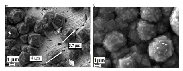
Figure 5 SEM images of diamond film on the stage of roughening of the globules structure (a) and their coating with numerous edges {100} (b)
