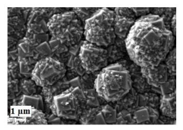
Figure 8: SEM images of diamond film on the stage of renucleation
