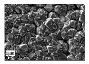
Figure 7 SEM images of diamond film on the stage of secondary formation of conic textures <110> and <111>
