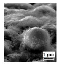
Figure 2: SEM image of diamond film on the globular stage
