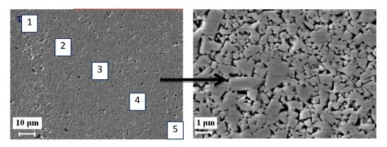
Figure 1: SEM image of the surface tungsten carbide of after a three-stage etching
