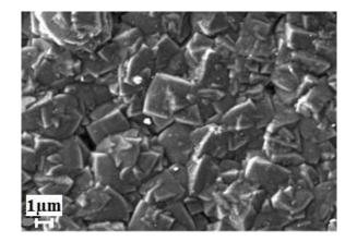
Figure 6: SEM images of diamond film on the stage of geometric selection
