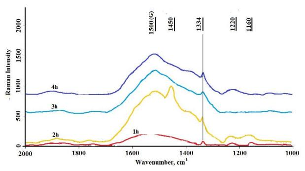
Figure 8: Raman spectroscopy of diamond film
