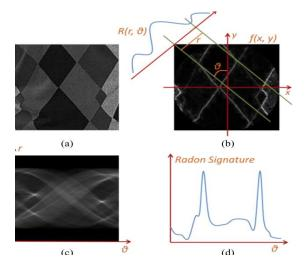
Fig.3. (a) an intensity image of clothing pattern. (b) Radon transform performed on a maximum disk area within the gradient map (c) Result of Radon Transform. (d) Feature vector of Radon Signature.
