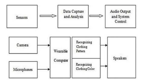
Fig.5.Block Diagram for cloth pattern using SURF
