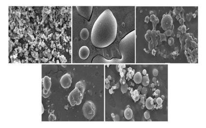
Figures 1: Morphology of (a) intact efavirenz, (b) PVP K-30, (c) Solid dispersion at ratio 2:1, (d) Solid dispersion at ratio 1:1 (e) Solid dispersion at ratio 1:2
