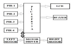
Figure 8: Block diagram of proposed system
