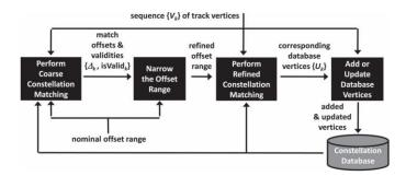
Figure 1: High level block diagram for updating a constellation database with a sequence of track vertices [5].
