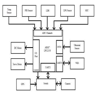
Figure 5: Robot Section [9]
