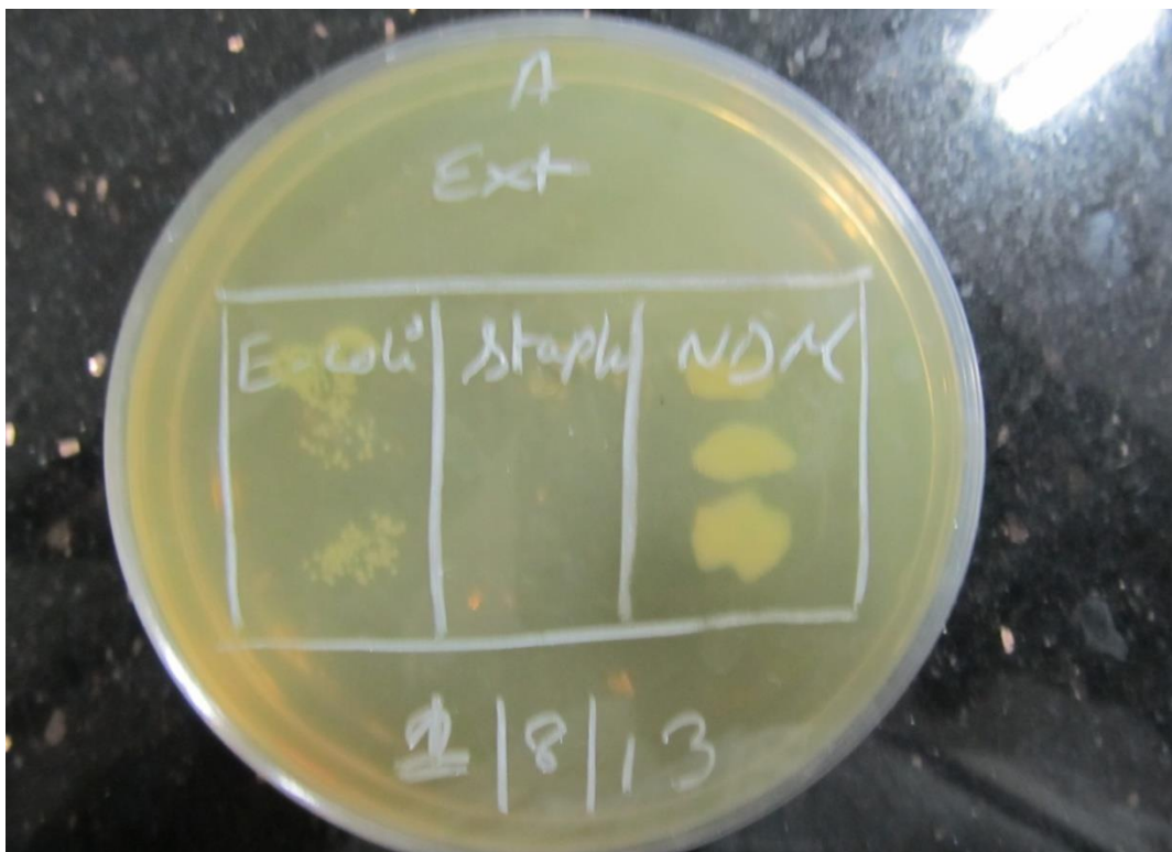
Fig.7. LELC showing minimum inhibition of E. coli , Staphylococcus aureus and nil inhibition of MDM strains by agar dilution method.
