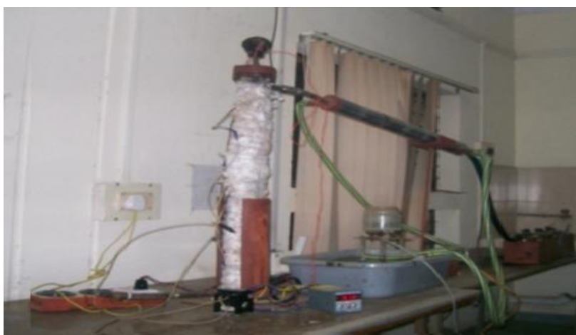
Figure 1: Experimental set up of pyrolysis reactor
