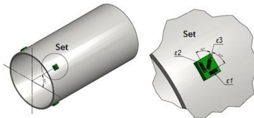
Figure 3: Scheme of placement of relative deformation sets relatively to a surface of a pipe
