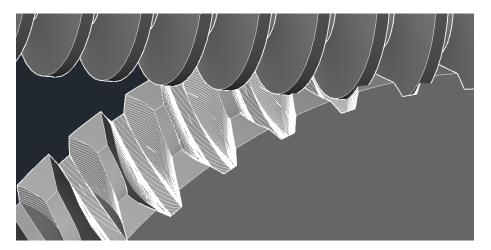
Figure 5: Shaping of worm wheel tool flank
