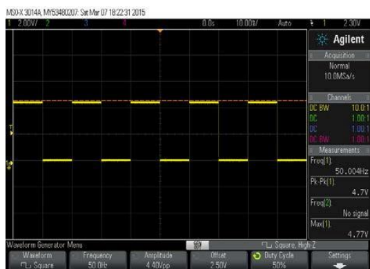
Figure 4: PWM output for 50% on time and 50% off time
