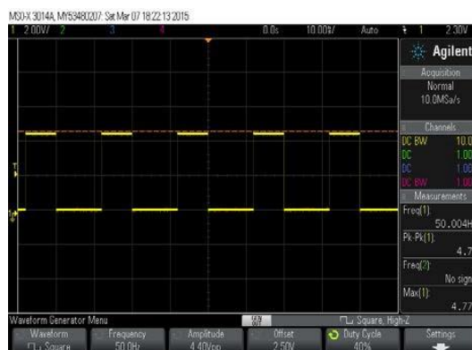
Figure 3: PWM output for 30% on time and 60% off time
