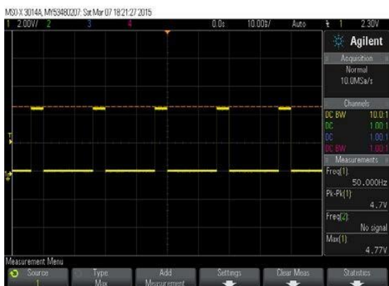
Figure 2: PWM output for 10% on time and 90% off time
