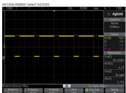
Figure 5: PWM output for 90% on time and 10% off time
