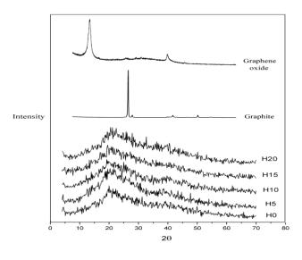
Figure 14: XRD pattern of graphite, graphene oxide and GOCH.
