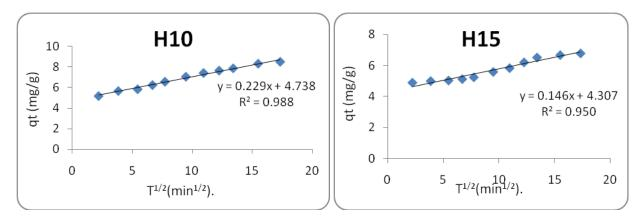
Figure 31: the relation between qt (mg/g) versus square root of contact time  $t^{1/2}$  (min<sup>1/2</sup>) of crosslinked GO/chitosan (H10)
