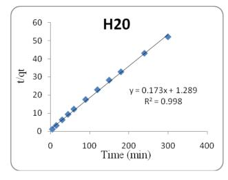
Figure 28: the relation between t/qt versus time t (min) for crosslinked GO/chitosan composite (H20)
