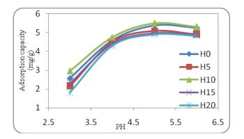
Figure 15: effect of pH value on the adsorption capacity GOCH.
