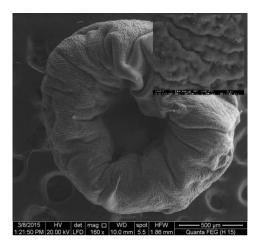
Figure 7: SEM micrograph of GO chitosan composite (H15)
