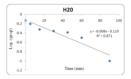
Figure 23: the relation between time t (min) and Log(qe-qt) for crosslinked GO/chitosan (H20)
