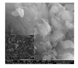
Figure 2: HR-SEM micrograph of GO powder
