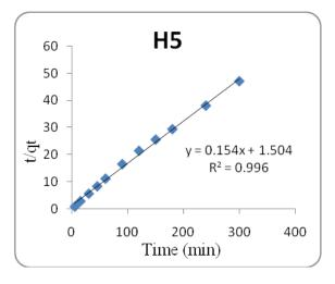
Figure 25: the relation between t/qt versus time t (min) for crosslinked GO/chitosan composite (H5)
