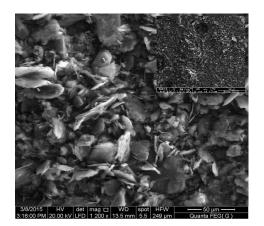
Figure 1: HR-SEM micrograph of graphite powder
