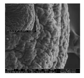
Figure 6: SEM micrograph of GO chitosan composite (H10)
