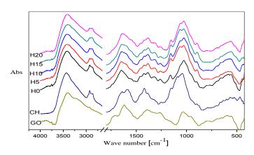
Figure 12: FT-IR spectra of GO, Chitosan Powder (CH) and GOCH.
