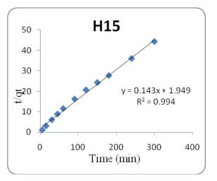
Figure 27: the relation between t/qt versus time t (min) for crosslinked GO/chitosan composite (H15)
