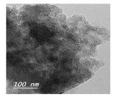
Figure 11: TEM micrograph of GO chitosan composite (H20)
