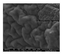
Figure 5: SEM micrograph of GO chitosan composite (H5)
