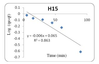
Figure 22: the relation between time t (min) and Log(qe-qt) for crosslinked GO/chitosan (H15)
