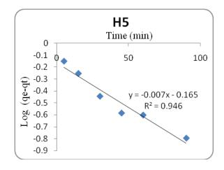
Figure 20: the relation between time t (min) and Log(qe-qt) for crosslinked GO/chitosan (H5)
