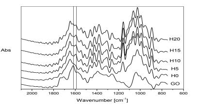
Figure 13: Deconvoluted FT-IR spectra of GO and graphene oxide crosslinked chitosan beads.
