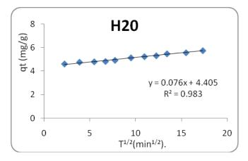
Figure 33: the relation between qt (mg/g) versus square root of contact time  $t^{1/2}$  (min<sup>1/2</sup>) of crosslinked GO/chitosan (H20)
