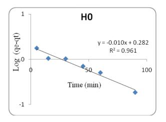
Figure 19: the relation between time t (min) and Log(qe-qt) for crosslinked chitosan (H0)
