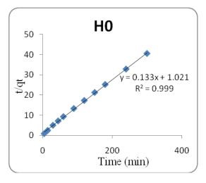
Figure 24: the relation between t/qt versus time t (min) for crosslinked chitosan (AH0)
