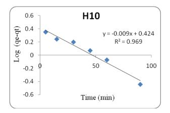
Figure 21: the relation between time t (min) and Log(qe-qt) for crosslinked GO/chitosan (H10)
