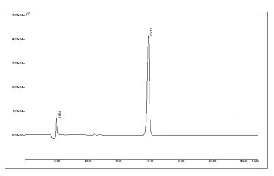
Figure 2: Chromatogram of torsemide in acid degradation [acid degraded product (2.033) and torsemide (7.933)]
