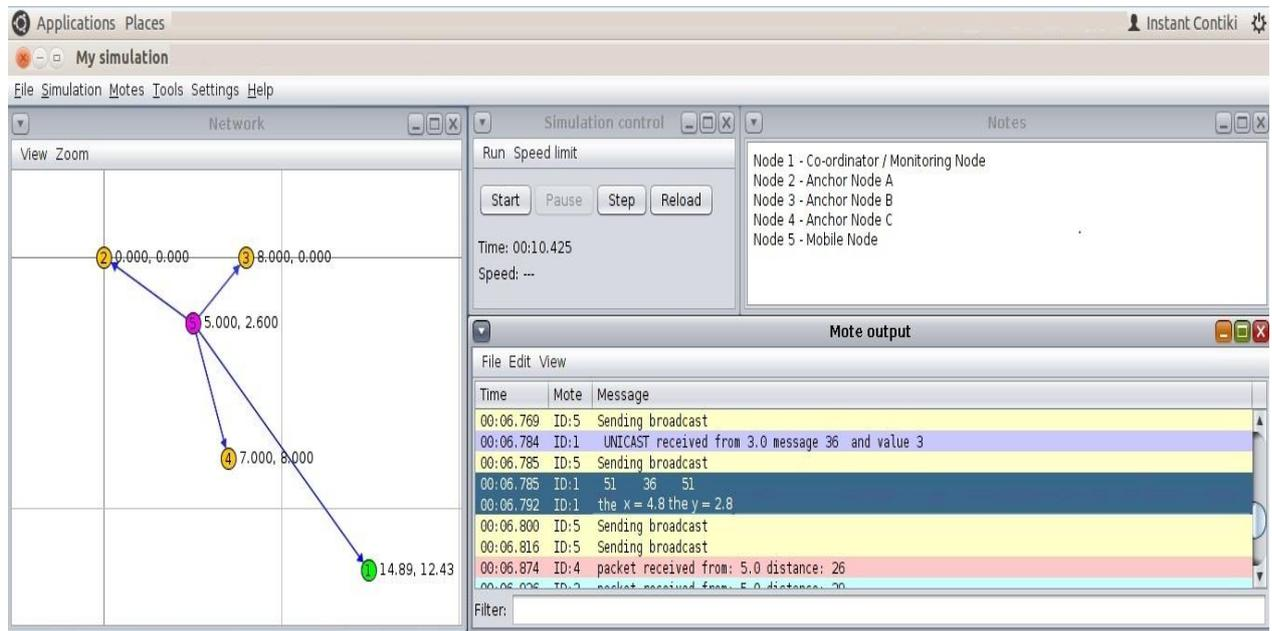
**Figure 6: Simulated Result - The Location of the mobile node estimated Using RSSI and Trilateration**
