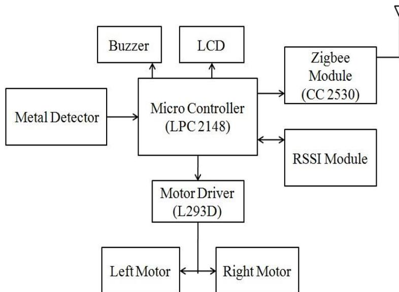
**Figure 1: Block Diagram of the Mobile Robot**
