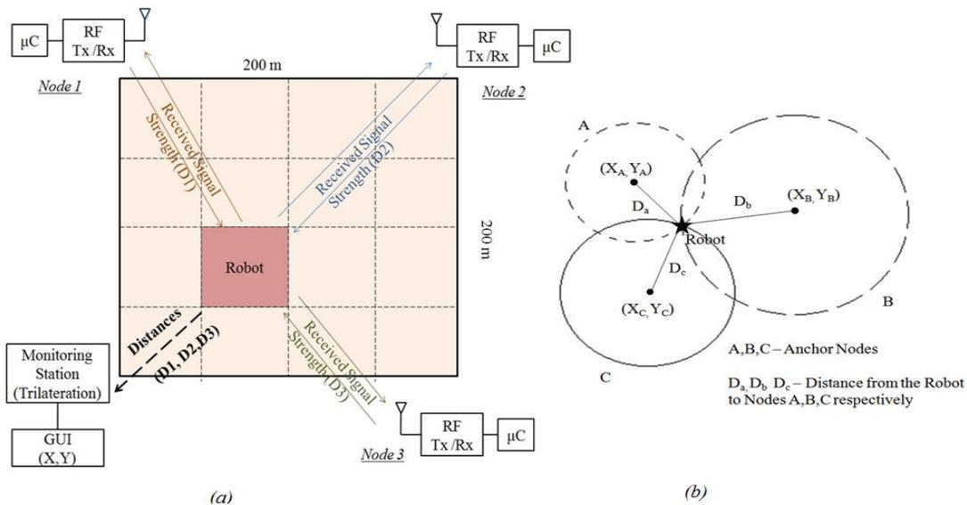
Figure 3: a) Distance Calculation using RSSI with three Anchor nodes
