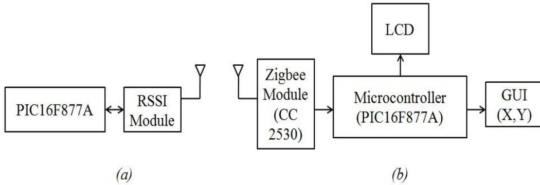
Figure 2: Block Diagram (a) The Anchor Nodes (1, 2, 3) (b) Remote Monitoring unit
