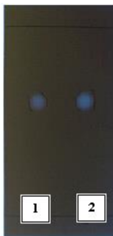
Figure 1: Thin-layer chromatograms of scopoletin under the UV light 365 nm (1. Scopoletin isolated from noni fruit; 2. Scopoletin comparator)
