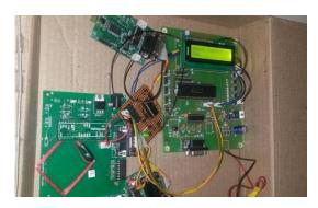
One side of the module contains the biomedical sensors to sense the various parameters and the other side sends the data to the imed box module through Zigbee. A buzzer is also connected to alert the patient to take medicine at proper time.
