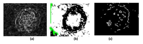
Figure 4: Segmentation results of the images (a) Gradient magnitude of the image (b) Segmented image (c) Image with its edge detected.
