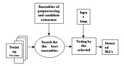
Fig.2. Block Diagram Of The Ensemble-Based Framework
