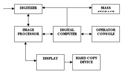
Fig 1 Block Diagram For Image Processing System
