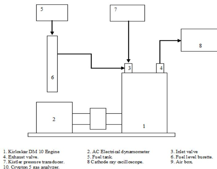
Figure 3: Schematic Diagram of Experimental Setup
