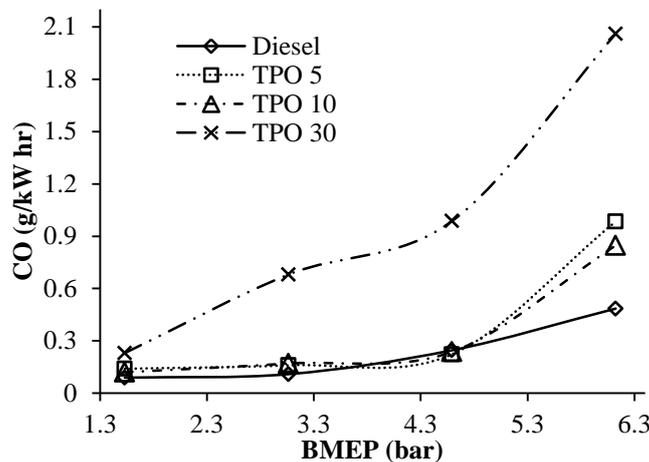
Figure 10: Variation of Brake Mean Effective Pressure with Carbon monoxide Emissions
