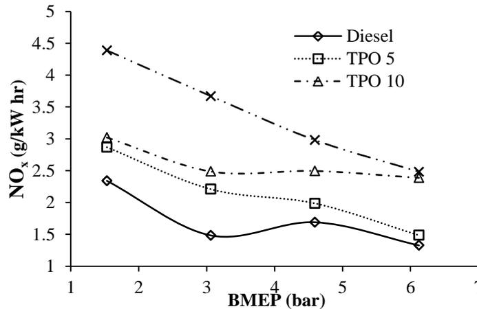
**Figure 9: Variation of Brake Mean Effective Pressure with Oxides of Nitrogen Emission**
