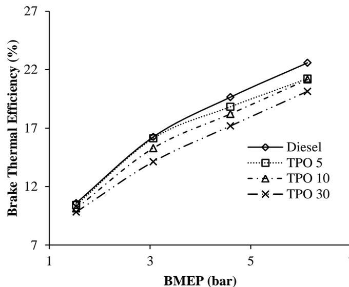
Figure 7: Variation of Brake Mean Effective Pressure with Brake Thermal Efficiency
