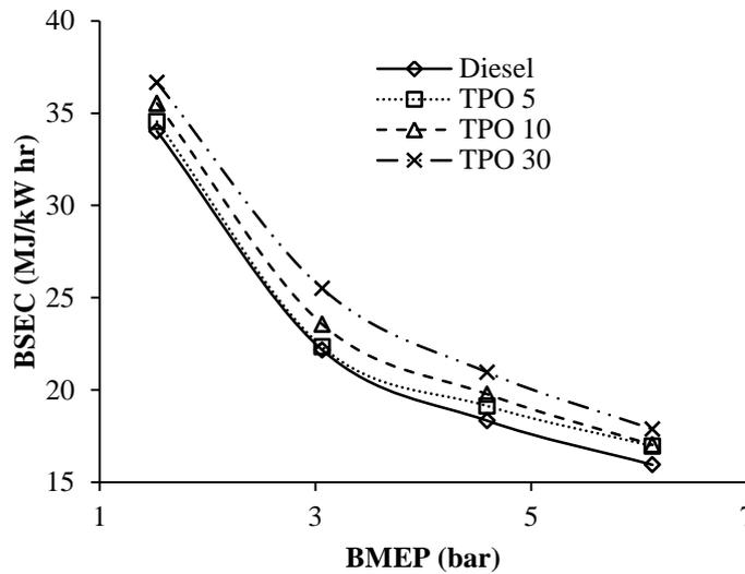
Figure 6: Variation of Brake Mean Effective Pressure with Brake Specific Energy Consumption
