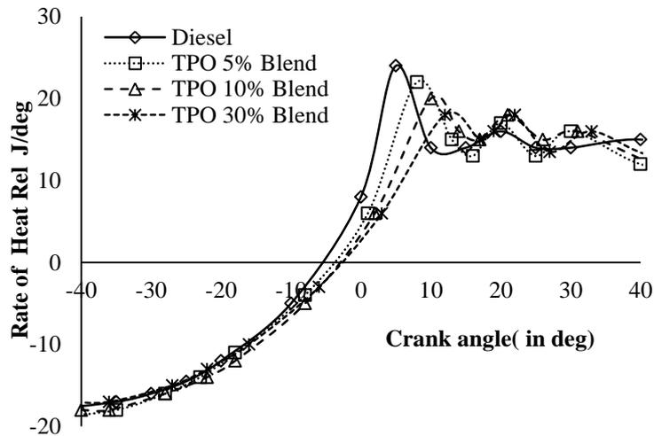
**Figure 5: Variation in Heat Release rate for Diesel and TPO blends at full load condition**
