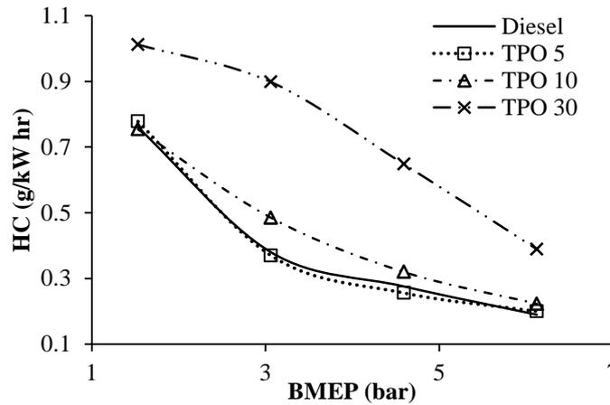
**Figure 8: Variation of Brake Mean Effective Pressure with Hydro carbons emission**
