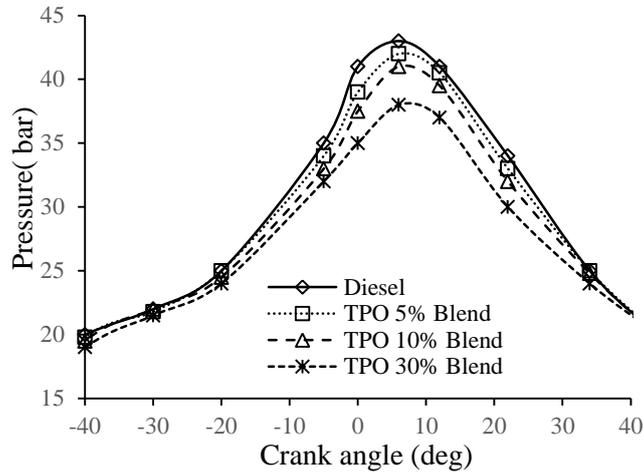
**Figure 4: Variation in In-Cylinder pressure for Diesel and TPO blends at full load condition**
