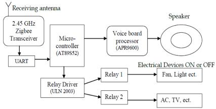
Figure 6: Sequence of operation of Receiving Module
