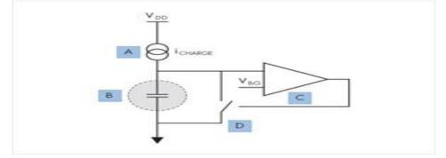
A - Current source; B - Sensor capacitor; C – Comparator; D - Discharge switch
