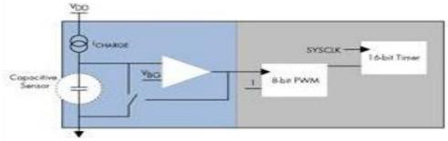
Figure 3: Capacitive Sensing Circuit
