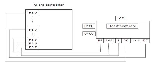
Figure 5: Interface circuitry for Heart beat rate display on LCD with Microcontroller
