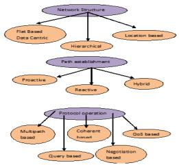
Figure 1: Grouping of Routing Protocols in WSN.
